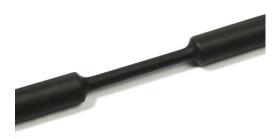
Heat Shrink Tubing, 4' Long Stick, Adhesive Lined, 3:1 Shrink Ratio, 1/2", 12.0/4.0 Dia, PO, Black, 10/pkg
